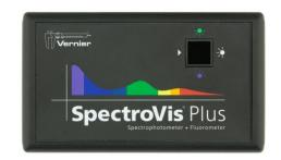
When measuring the absorbance, insert the cuvette into the shaft of the spectrometer – in the picture the shaft opening is in the top right corner. To the right of the shaft there is a mark of a white light source (white circle with rays). The light shines through the cuvette; each individual wavelength is absorbed to a different degree. Photons continue towards the detector (in the picture marked by a white triangle).
